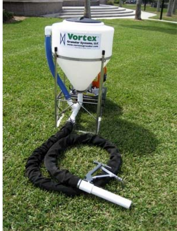
Figure 3. TR Vortex system to be used for SediMite application
