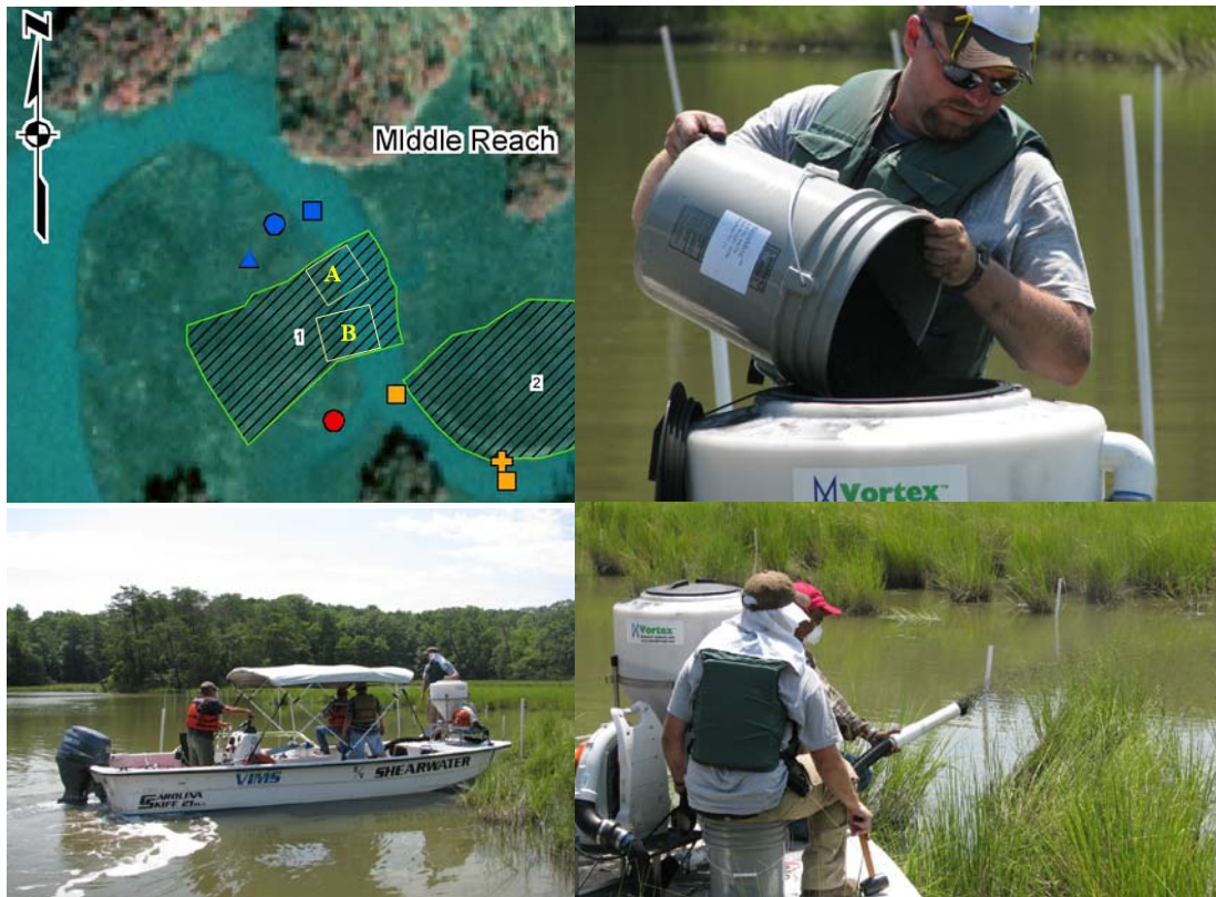
Figure 5. Top left: position of treatment areas aligned along the edge of the Creek. Remaining pictures show deployment on a boat and application using the Vortex device for application of SediMite in the estuarine wetland at Ft. Eustis.
