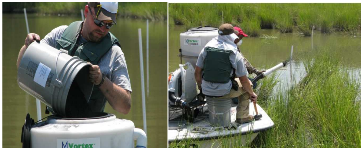
Figure A3. Application of SediMite™ in a contaminated tidal wetland using an air blown applicator minimizes adverse impacts to existing vegetation and benthic organisms while reducing contaminant uptake in the food chain.
